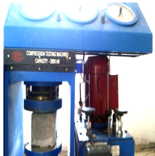
Fig. 2. Testing of cube specimens in compression.
