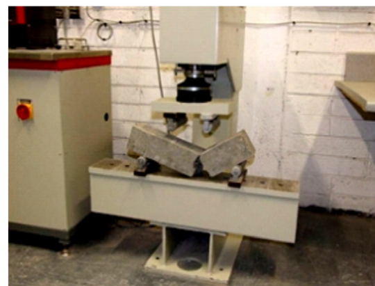
Fig. 3. Testing of beam specimens in flexure.
